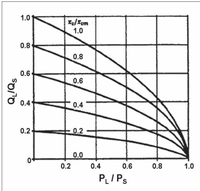
Figure 2. Change in the load flow with the valve displacement and the load pressure.
