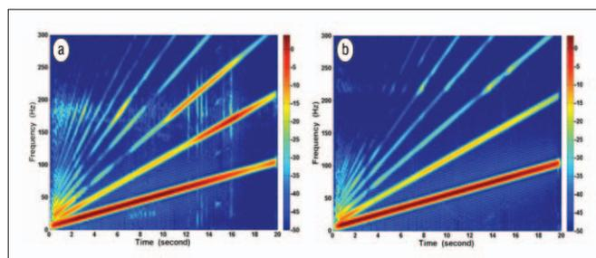
Figure 11. Frequency-time representation of the weighted-sum ground force from 5–105 Hz. (a) Model 362. (b) Model 364.
