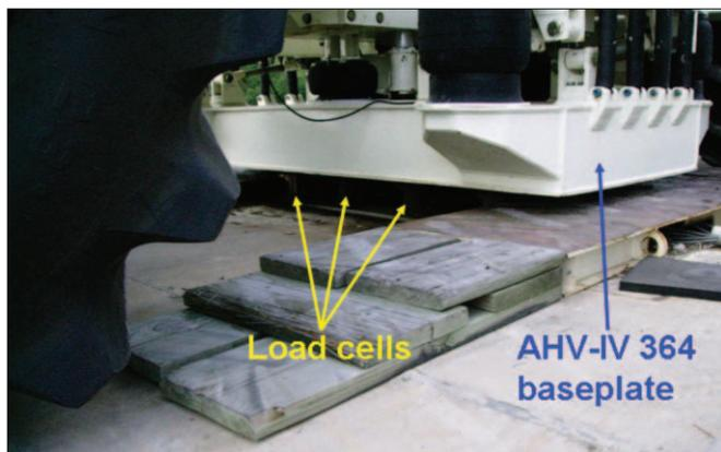
Figure 9. Model 364 on load cells.
