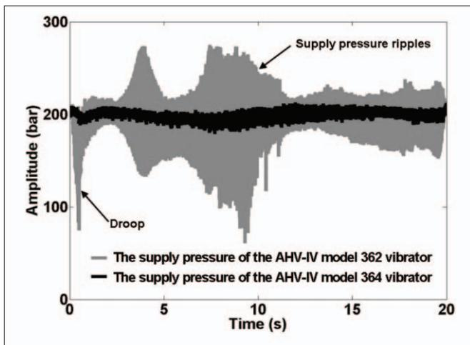
Figure 7. The hydraulic supply pressures of the AHV-IV vibrators.
