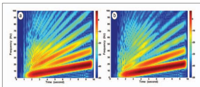
**Figure 6.** Comparisons of the ground force measured by load cells at frequencies of 1–21 Hz. (a) Nonlinear control off. (b) Nonlinear control on.
