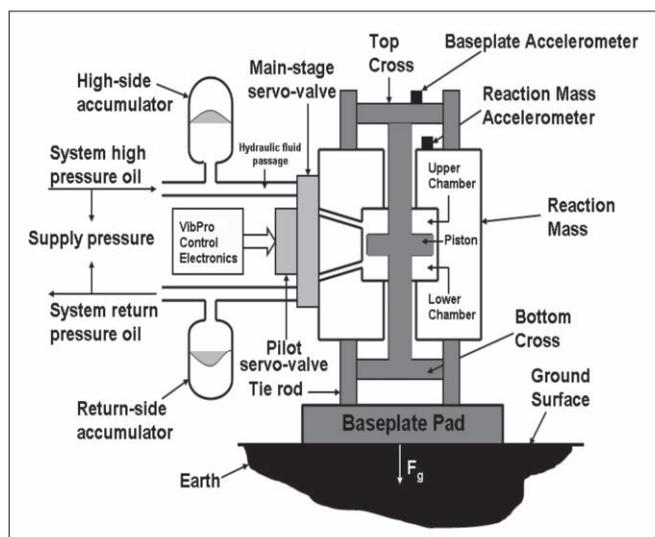
Figure 1. Schematic of an AHV-IV vibrator.
