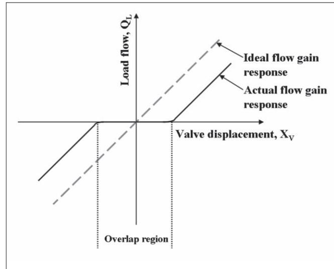
Figure 3. Load flow gain and overlap of the main-stage valve.
