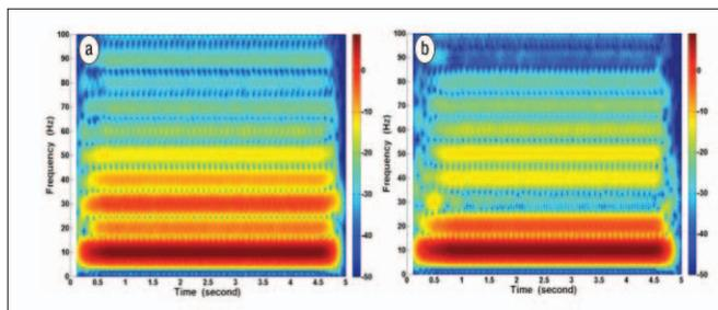
**Figure 5.** Comparisons of the ground force measured by load cells. (a) Nonlinear control off. (b) Nonlinear control on.
