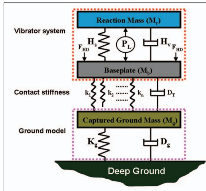
Figure 8. The vibrator-ground model.
