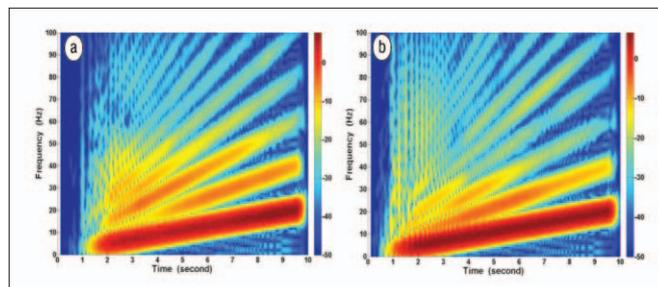
Figure 10. Frequency-time representation of the weighted-sum ground force from 1–21 Hz. (a) Model 362. (b) Model 364.
