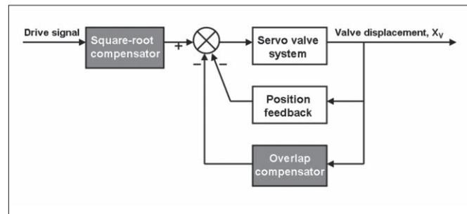
Figure 4. Nonlinear control block diagram.
